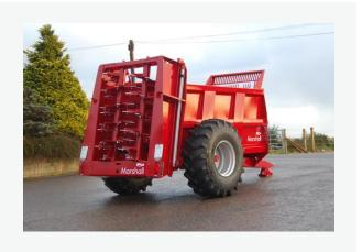
**ALWAYS** close the slurry door after spreading, this firstly protects the ram and avoids unnecessary stress on the door slides when travelling.
